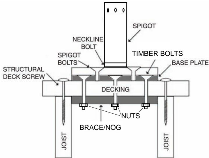
1. To fix spigot to timber deck – You will need four 10X150mm stainless countersunk bolts or similar. Attach these bolts through suitable braces or nogs securely fixed between the deck joists or beams.
